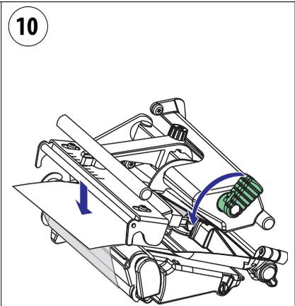
*Turn the printhead lift lever counter-clockwise to engage the printhead.*
