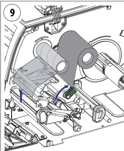
Turn the printhead lift lever clockwise to raise the printhead and release the ribbon.
