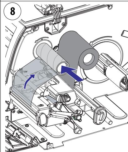
Slide the empty cardboard core onto the ribbon rewind hub so the ribbon is wound up when the hub rotates counterclockwise.
