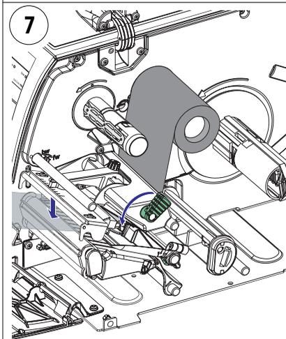
Without releasing the ribbon, turn the printhead lift lever counterclockwise to engage the printhead and lock the ribbon.
