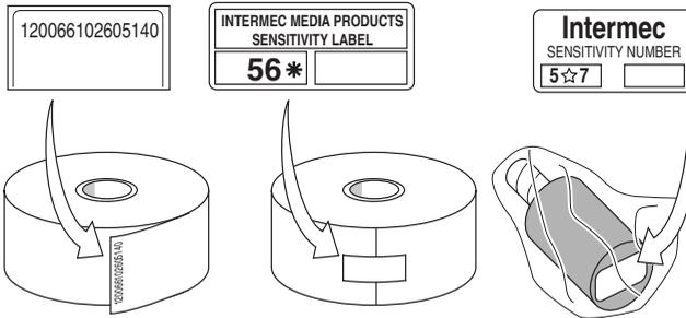
Use this three-digit number to optimize print quality and print speed on your printer. You can achieve the best print quality on the printer by using Intermec ribbon and media products.
