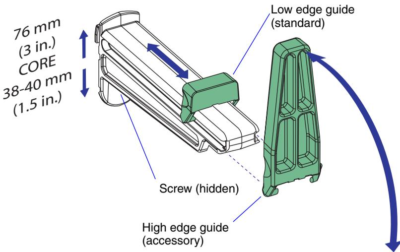
Optionally, the printer can be fitted with an 1.5-inch rotating media supply hub instead of a post and a paper sensor, which detects when the remaining amount of media has reach a level specified in the Setup Mode. There are also a 3-inch adapter and a label roll retainer. Another option is an internal guide for media placed behind the printer (for example fan-folds). For illustrations, see Chapter 8 “Options”.
