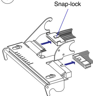
Disconnect the cables from the printhead. Note the snap-lock on the inner connector. Pull at the connectors—not at the cables!
