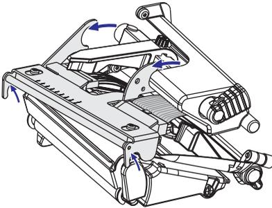
Disconnect the printhead bracket from the print mechanism as indicated by the arrows and pull out the printhead as far as the cables allow.
