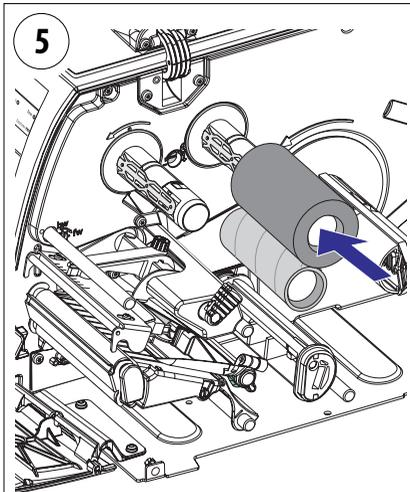
Slide the ribbon roll onto the supply hub so the ink-coated side faces down when the ribbon is routed through the print mechanism.
