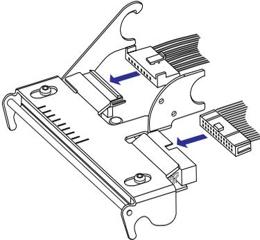
Connect the two cables to the replacement printhead.
