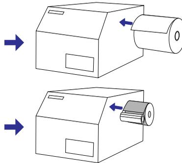
Allow the cleaned parts to dry before loading any media (and ribbon).
