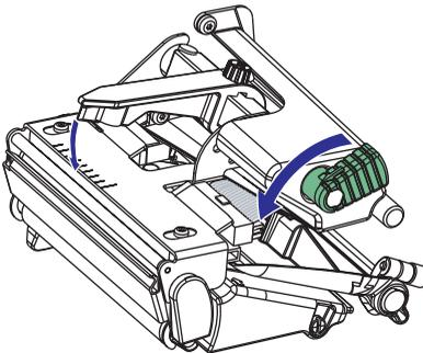
Turn the printhead lift lever counter-clockwise so the magnet engages the printhead bracket.
