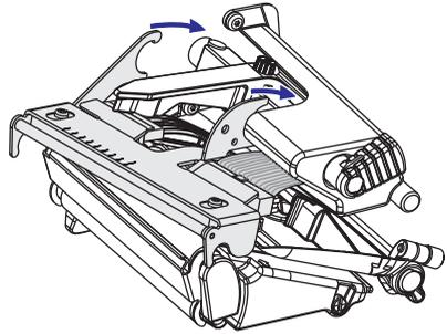
Put back the printhead in reverse order and check that the printhead cables run freely.
