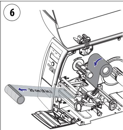
Route the ribbon through the print mechanism underneath the transparent upper LSS guide and pull out approximately 20 cm (8 inches) of ribbon leader.
