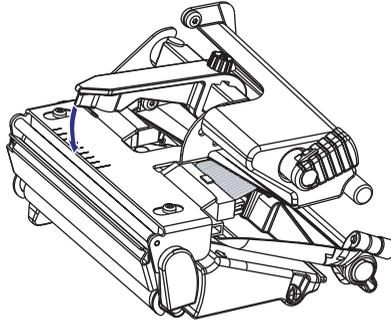
Pull the printhead bracket away from the magnet in the pressure arm.
