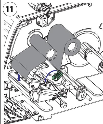
Turn the printhead lift knob counter-clockwise to engage the printhead.
