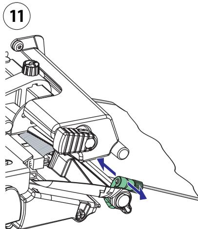
*Adjust the position of the green edge guide so the media is guided with a minimum of play. Lock with the nut.*
