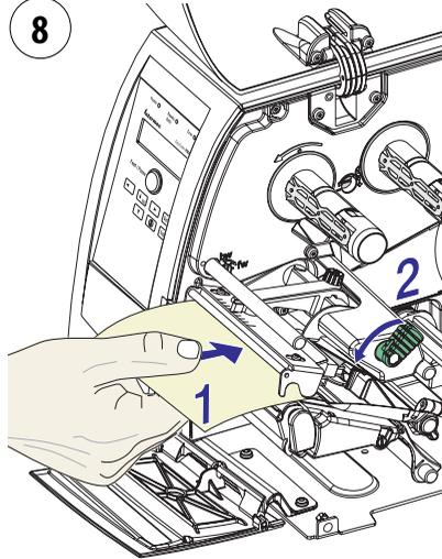
Insert most of the cleaning card under the printhead again (1). Engage the printhead (2).
