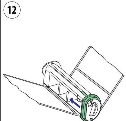
*Adjust the position of the edge guide on the label slack absorber according to the width of the media.*
