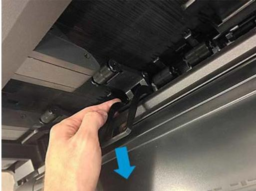
2. Push the stacker wheel lifter's left leg to unclip it. Be sure not to unclip the second wheel holder.
