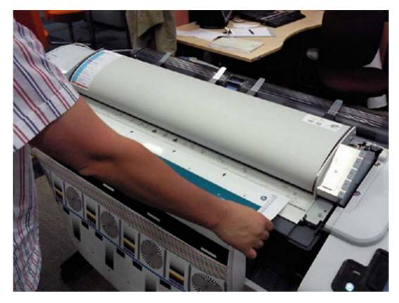
9. Follow the next steps to calculate the Y-Axis adjustment scale: Measure the total length of the two vertical rules at both sides of the copied plot (we call it M1 and M2).
