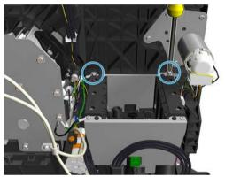
4. Remove the bracket and side plate.
