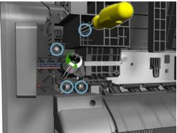
5. Remove the stacker, pulling the handles on the back.
