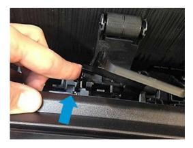
When the left leg is unclipped, the right leg will come out too. Remove each stacker wheel lifter.
