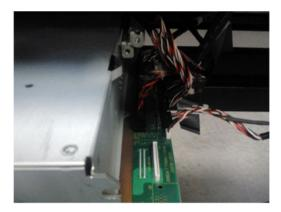
Remove the E-Box from the printer.
