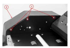
Remove the screws (1), and then the motor cover (2).
