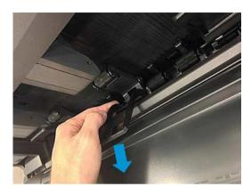
Push the stacker wheel lifter's left leg to unclip it. Be sure not unclip the second wheel holder.
