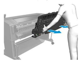
NOTE: For installation make sure that the valves are down and the ramps are hidden, otherwise it can cause improper assembly, and show SE90:03 or SE89:03.
