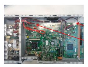
3. Unroute the cables and remove one T-10 screw.
