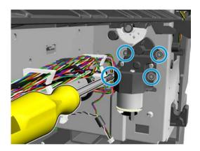
4. Remove the valves motor.
