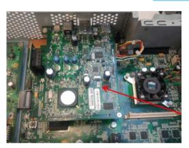
4. Remove the two screws shown.
