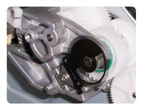
Press the encoder using the Media Advance Drive Adjustment Tool (reversed) so that it sticks to the
