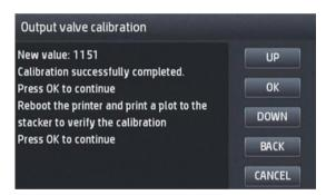
5. By pressing **OK** in the next screen, the printer will shut down automatically.
