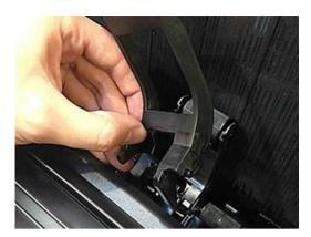
Before assembling the MFP stacker wheel lifters, check the following reference images for guidance: The hook of the stacker wheel lifter for MFP should be inserted into the hole shown by the blue arrow.
