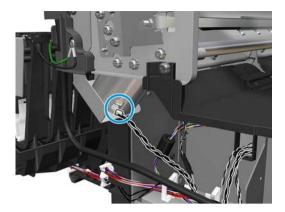
6. Remove the 2 screws in order to remove the piece.
