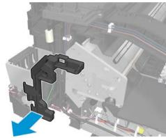
7. Remove the screw in order to remove the metallic piece.
