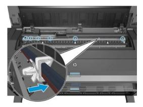
4. Remove 2 T-20 screws, and the second starwheel rail.
