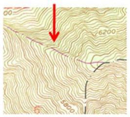
Streaks running in the scan direction which seem to appear and disappear during the scan aremost likely caused by dust. Clean the scanner and the original. The streaks are often a darker shade of color.
