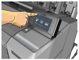
The front panel is located on the front right of the printer. It gives you complete control of your printer: from the front panel, you can print, view information about the printer, change printer settings, perform calibrations and tests, and so on. The front panel also displays alerts (warning and error messages) when necessary.
