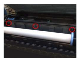
Unhook the 2 hooks, and remove the bumper.
