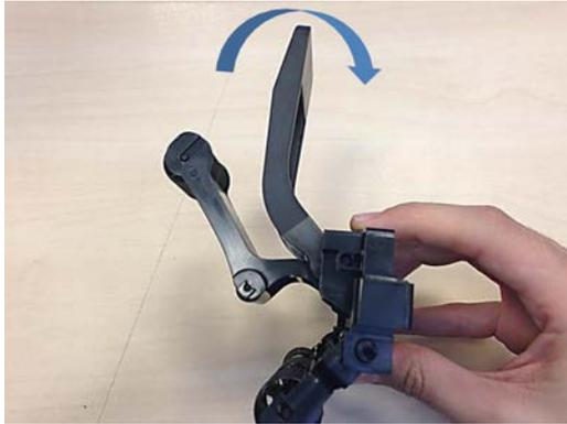
2. Press the right leg of the stacker wheel lifter to unclip it.
