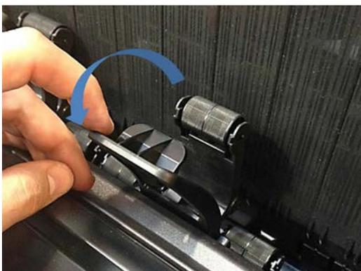
5. Attach the hinge stoppers on both sides. Each hinge stopper is attached to the stacker with one screw.
