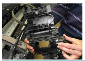
NOTE: When assembling the belt, make sure that it is correctly attached to the tensioner and scan axis motor pin. If not,the belt can rapidly become worn out, and/or make noise.
