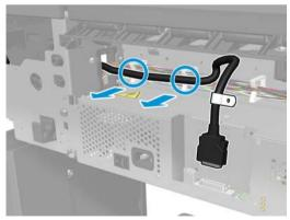
6. Remove the screw, pull the cable through the hole, and unclip it.
