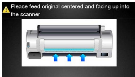
8. The Control Panel prompts you to feed the original. Load the Scanner IQ plot that you printed previously in the Scanner input tray. Wait then for the product to scan and print the image.
