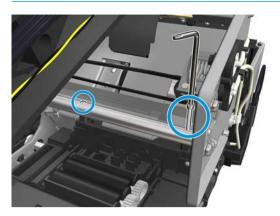
Remove the 2 T-15 screws and the left bracket.
