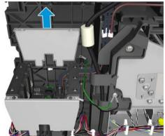
5. Remove 2 screws and the side plate.
