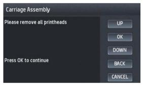
If the printheads were not correctly removed after pressing the **OK** button, a message appears asking to remove them. To do so, repeat the previous steps. If the printheads were correctly removed (it is clear there are no printheads installed in the carriage), and the message still appears, press the Cancel (X) key; the test will finish, and the appropriate error code will appear.
