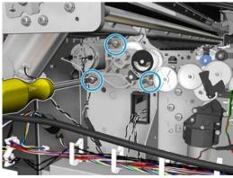
**7.** Remove the paper axis motor.
