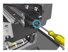
3. Remove the bump cutter actuator.
