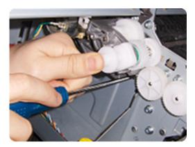
While maintaining pressure on the Media Advance Drive Adjustment Tool, fully tighten the encoder sensor adjustment screw.
