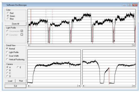
The Adjusted light profile is corrected according to the calibration sheet, in other words, the calibration sheet has been used as a reference to correct the imperfection of the CIS elements.
