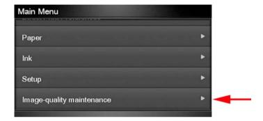
From the Image-quality maintenance menu, scroll down and select the Scanner IQ plot to print.
