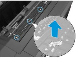
5. Lift up the flap at both sides and remove the overdrive.
