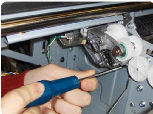
3. Loosen the encoder sensor adjustment screw.
