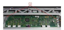
Unclip the USB Cable and pull it gently out of the CIS bridge (1). Remove the screws and unclip the cable
