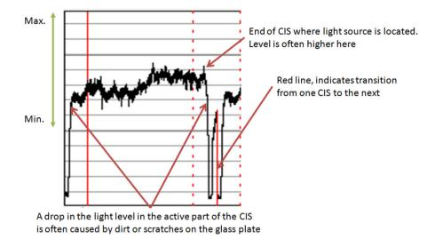
A white patch is located at each end of the CIS element. The one at the start of the CIS is a bit smaller than the one at the end, it makes a black point, unlike the end which makes a Black and a White point.
