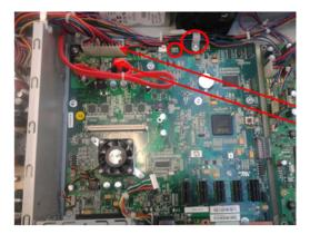
Remove four T-8 screws and the L-shaped metal sheet.
