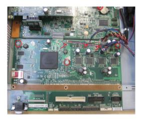
Slide out and remove the engine PCA (which is connected to the formatter PCA).
