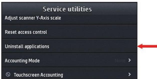
2. A message similar to the following will be displayed in the Front Panel. Press the **OK** button to remove the installed applications, or press **Back** or **Cancel** to exit.
