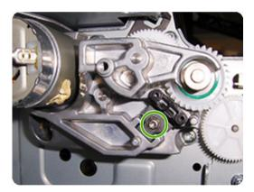
Insert the three T-15 attachment screws, but do not fully tighten them.
