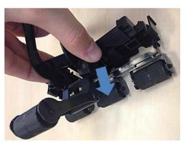
The stacker wheel lifter is now removed from the Hand-off assembly.
