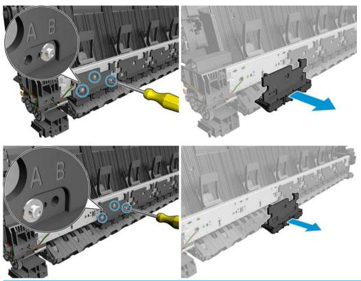
For installation make sure that you install the 1st pinch using hole B.
