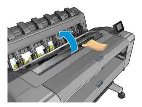
2. Move the carriage manually to the left side of the printer, if feasible.
