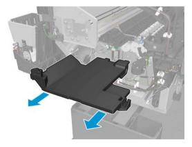
Remove the first starwheel rail. See <u>Customer Self Repair Flyers on page 389</u>.
