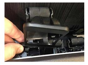
Push the stacker wheel lifter's left leg to align the left pin with the left groove.
