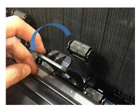
Attach the hinge stoppers on both sides. Each hinge stopper is attached to the stacker with one screw. **5.**
