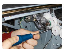
Loosen the encoder sensor adjustment screw.
