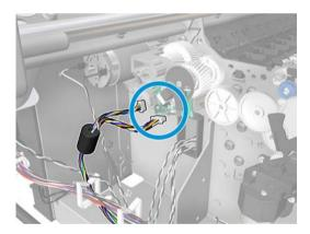
Remove the 2 screws and remove the connectors.
