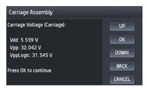
The diagnostic test will check the carriage LEDs and sensors. This can take some minutes. The following 5. message appears in the front panel:
