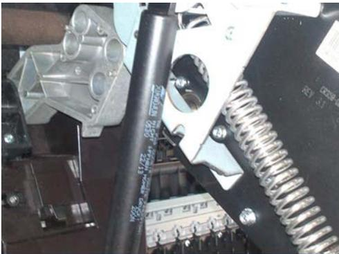
5. Remove the lift assembly. See [Lift assembly on page 376](#).
