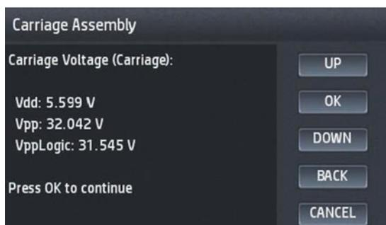
5. The diagnostic test will check the carriage LEDs and sensors. This can take some minutes. The following message appears in the front panel:
