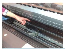
NOTE: An angle screwdriver is needed, if not, you will have to remove scanner covers (FP and SVS side).
