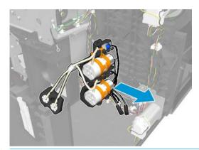
NOTE: The primer service kit includes the valves, the plastic, and the tubes.
