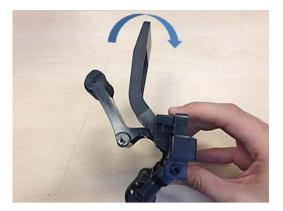
Press the right leg of the stacker wheel lifter to unclip it.
