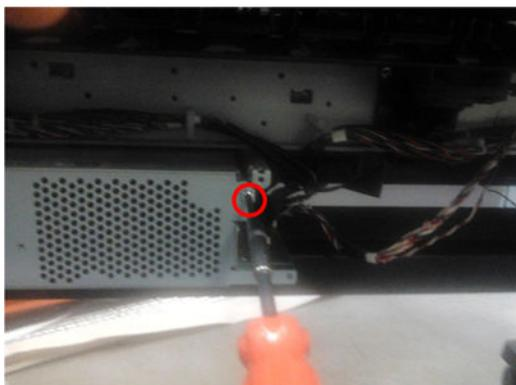
4. Remove the front panel cable and the T-10 screw. For the T2500 and T3500, you will also need to disconnect the USB cable.
