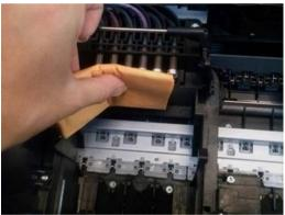
**d.** Try to close the carriage latch again. If necessary, push against the rear side of the carriage to ensure it is properly closed.
