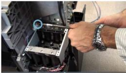
Remove the service station. See <u>Service Station with Drop Detector on page 268</u>.
