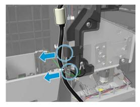
7. Remove the front panel screw.
