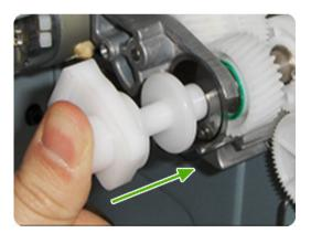
While maintaining pressure on the Media Advance Drive Adjustment Tool, fully tighten the three T-15 6. attachment screws in the order shown.
