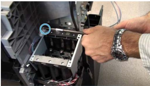
7. Remove the service station. See [Service Station with Drop Detector on page 268](#).
