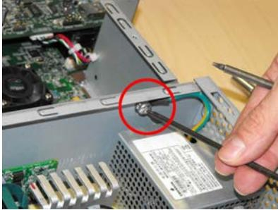
6. Remove the power supply unit.
