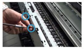
Remove the ISSWALL (removing 2 T-10 screws).
