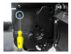
Remove 3 T-15 screws and the rewinder.
