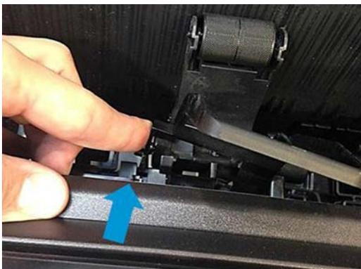
4. When the left leg is unclipped, the right leg will come out too. Remove each stacker wheel lifter.
