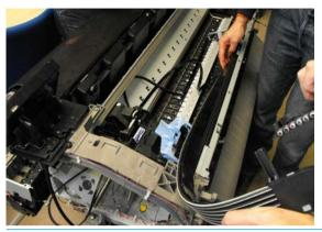
NOTE: After installing the carriage, when closing the latch, make sure the carriage is placed in the printhead replacement position so the carriage doesn't interfere with the rear guide.
