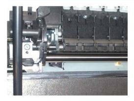
Remove the circlip.
