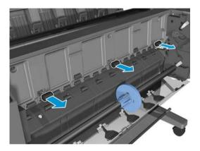
5. Remove the 3 T-15 screws underneath.
