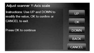
13. Press **UP** and **DOWN** to pre-set the new value of Y-Axis adjustment scale and press **OK**.
