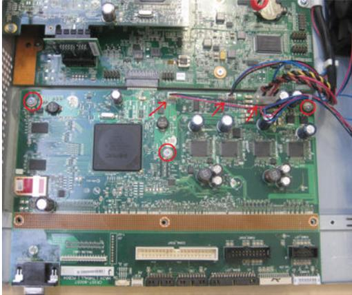
3. Slide out and remove the engine PCA (which is connected to the formatter PCA).
