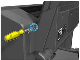
Remove the fixed tray cover from the front panel side.
