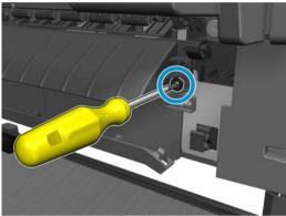
3. Remove the output platen.
