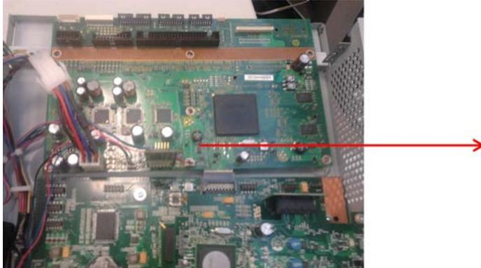
**⚠ WARNING!** If the engine PCA is not removed before the formatter, the bridge connections may be damaged.
