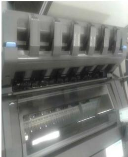
After printing with thin media, remember to return the blue lever so that there is a small gap between the arms and stacker tray.
