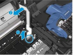
Unclip the mylar, and disconnect trailing cable.
