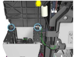
4. Remove the bracket and side plate.
