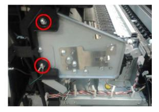
8. Remove the Scan Axis Motor. See Scan Axis Motor on page 264.
