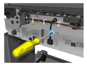
Disconnect and unclip the front panel cable.
