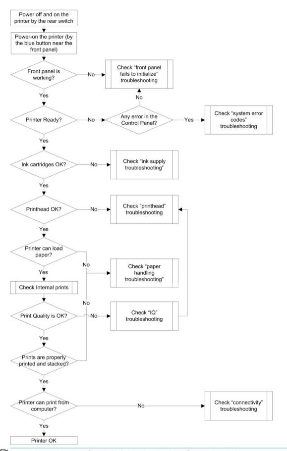
NOTE: Once an issue is confirmed, check that printer has latest firmware installed.
