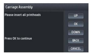
If the printheads were not correctly installed after pressing the **OK** button, a message appears asking to install them. To do so, repeat the previous steps. If on checking, the printheads were correctly installed (it is clear there are printheads installed in the carriage), and the message still appears, press the Cancel (X) key; the test will finish, and the appropriate error code will appear.
