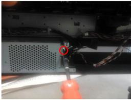
4. Remove the front panel cable and the T-10 screw. For the T2500 and T3500, you will also need to disconnect the USB cable.
