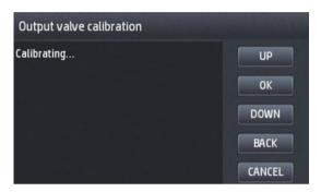
4. At the end of the process, you will have the result of the calibration. The screen will show also a recommendation to verify the calibration (print a plot to stacker). Typical values for the calibration range from 1015 to 1225.
