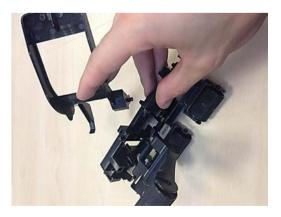
Assemble multi-function printer stacker wheel lifters
