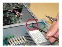
Remove the power supply unit.
