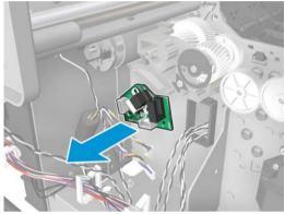
Disconnect the cable, and remove the 3 screws.
