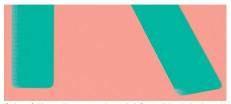
If edges of objects or lines appear to be poorly defined or lighter in density, and you have already set the print-quality slider to **Quality** in the driver dialog, select the custom print-quality options, and try setting the quality level to **Normal**. See users guide.
