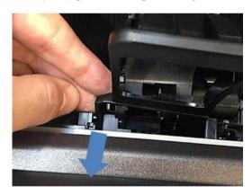
Check that the stacker wheel lifter can rotate freely.
