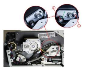
Remove the motor screws.
