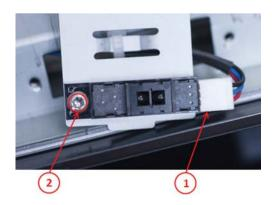
9. Squeeze lock pins, and remove the Lid Sensor.
