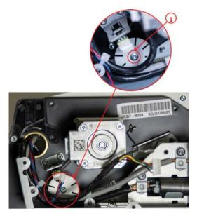
Release belt tension by loosening the screw (don't remove it), and push the tension wheel upwards and tighten the screw.
