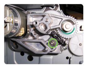
Add the Encoder Sensor Tool to the Media Drive Adjustment Tool.
