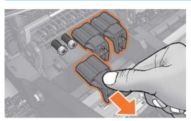
After inserting the printhead, the printer will check electronic connections. If the check fails, the printer will ask to reseat the printhead.
