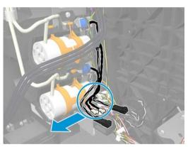
3. Remove the T-20 screw, the T-10 screw, the tubes, and the plastic pieces.
