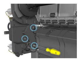
Remove the bottom rewinder support.
